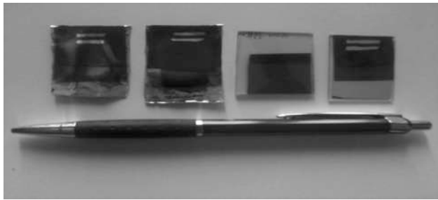
Fig. 5 Thin film solar cell fabricated by using 2D QPC
