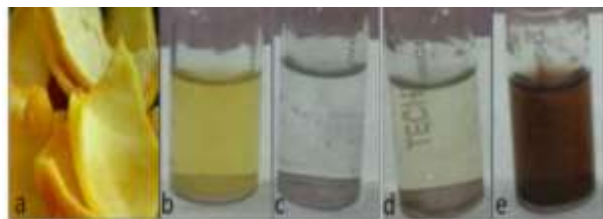
Fig. 1. Biosynthesis of AgNPs using MPs aqueous extract a) Musambi peels, b) Aqueous xtract of MPs, c) 1mM \text{AgNO}_3 , d) Reaction mixture 0 th min and e) Reaction mixture after 24h.
